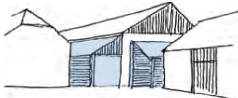
Smaller peripheral elements of building can reduce the bulk of the main element.
