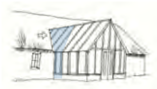
Cutting into roofline.
