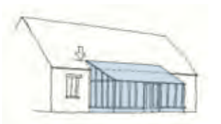
Overlapping eaves line.
