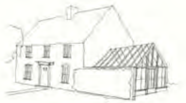
Screening to retain symmetry.
