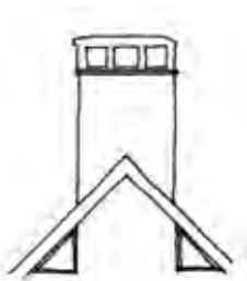
Combined flues and other service elements can be housed in roofline features.
