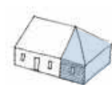
Additional bay with contrasting cladding.
