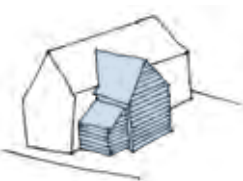
Secondary roof and lean-to.
